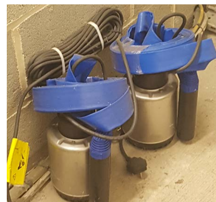
Two puddle pumps to help with the removal of water.
