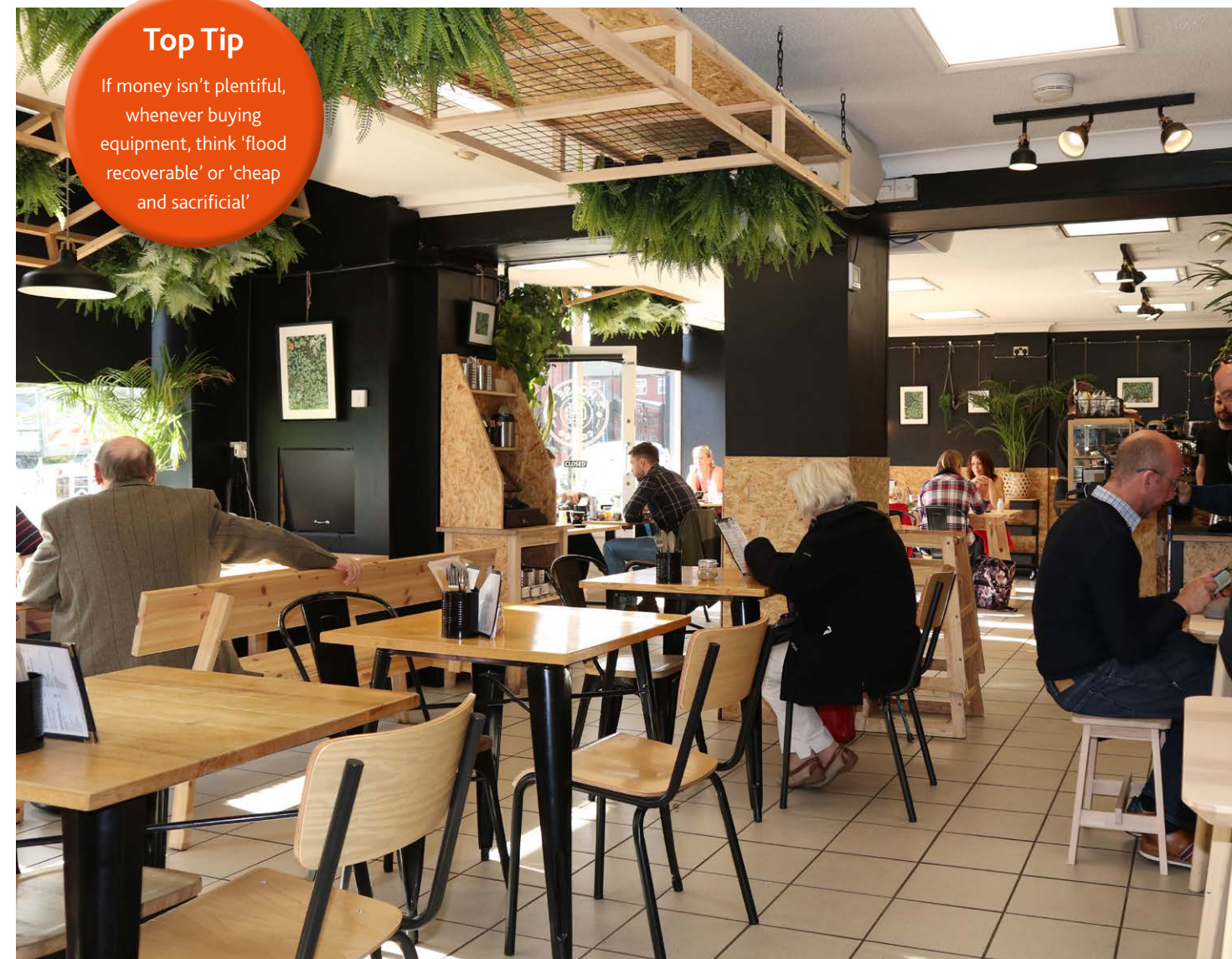
OSB boarding pinned to the wall can easily be removed and replaced to allow the walls behind to dry out.
